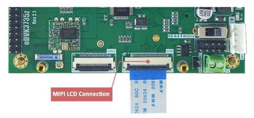
The eSOM3735z support both HDMI and MIPI LCD simultaneous with special Windows 10 that released for this board.
